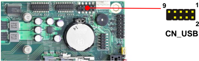
CN_USB: USB2.0 10-pin header (Pitch 2.54 mm)
