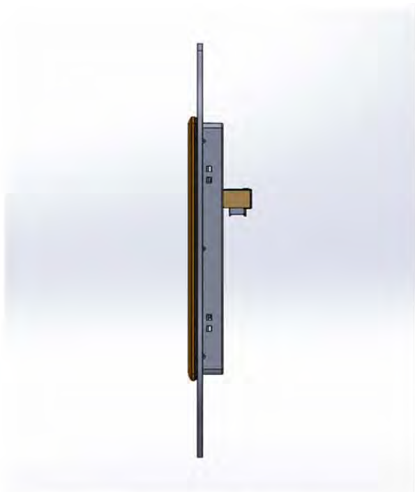
Panel mount side view with LVDS connector
