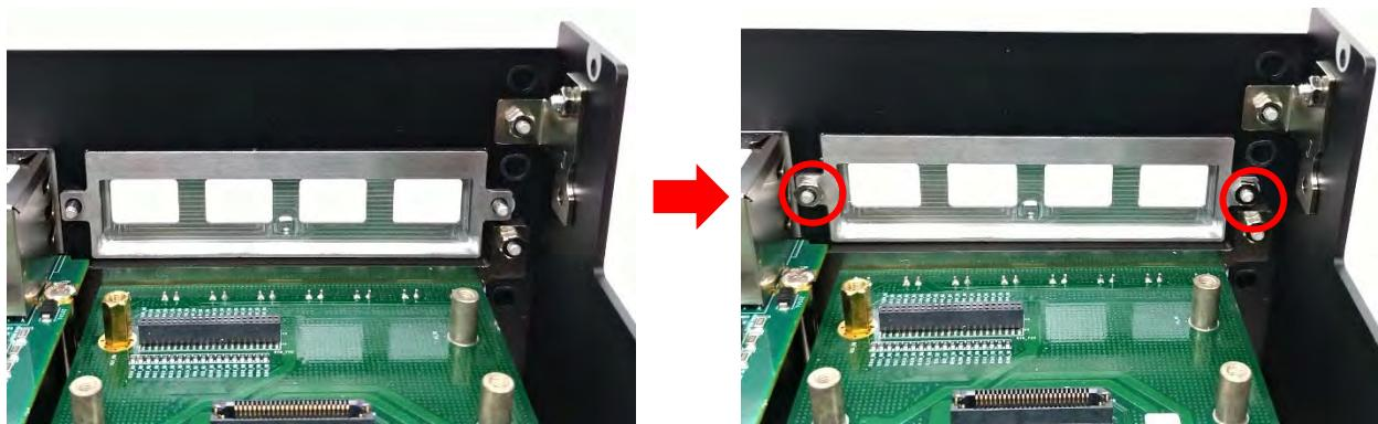
3. Locate the connector BTB\_FH1\_DB on DP-300 DTB.
