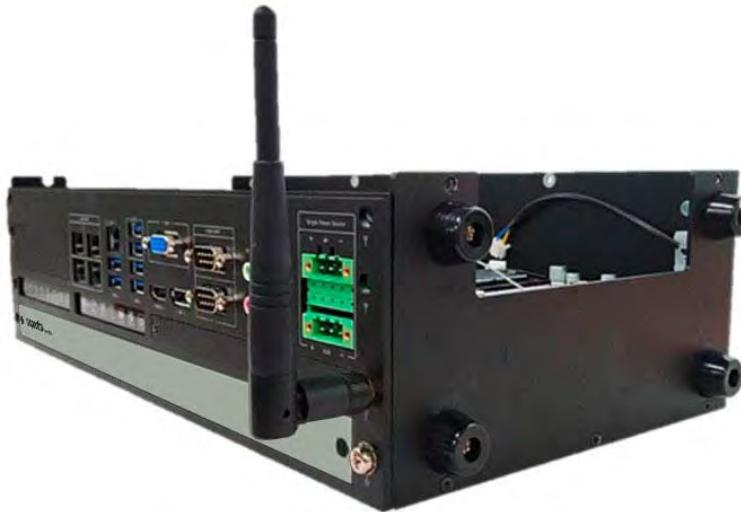
5. Attach the RF connector of the cable's another end onto the card.
