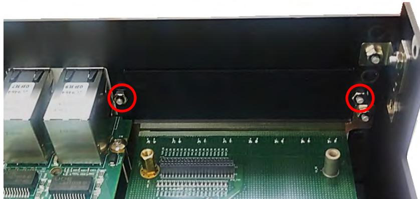
2. Attach the MEC-USB bracket, and fasten the 2 hex nuts to fix it as indicated.
