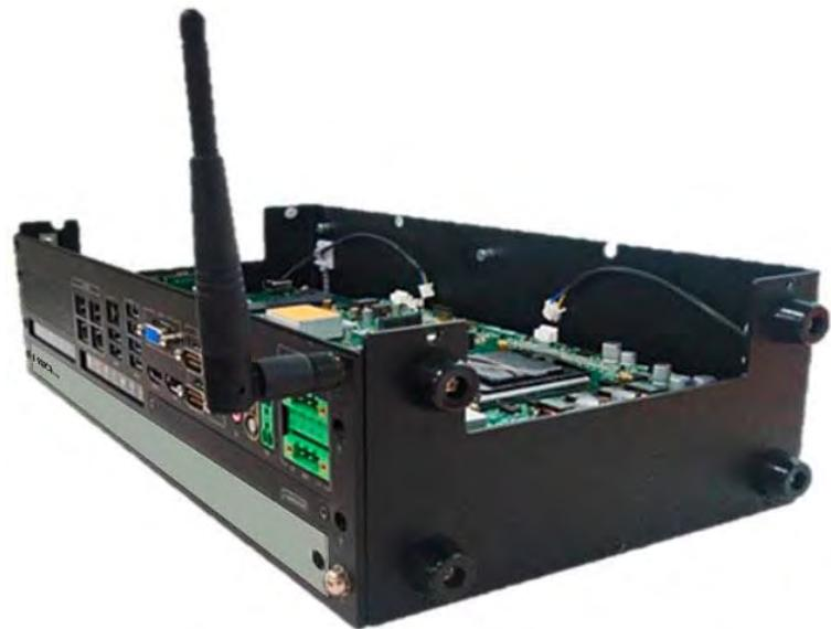
5. Attach the RF connector of the cable's another end onto the card.
