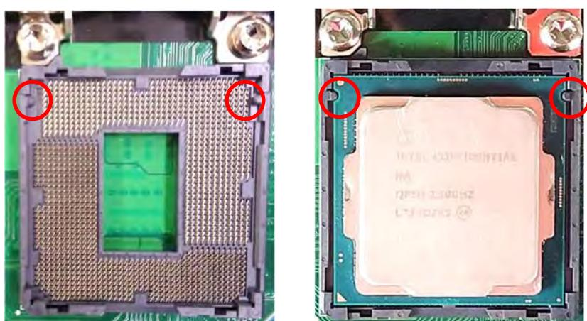
4. Place the thermal pad on the CPU heat spreader. Press down the socket lever to lock the CPU.
