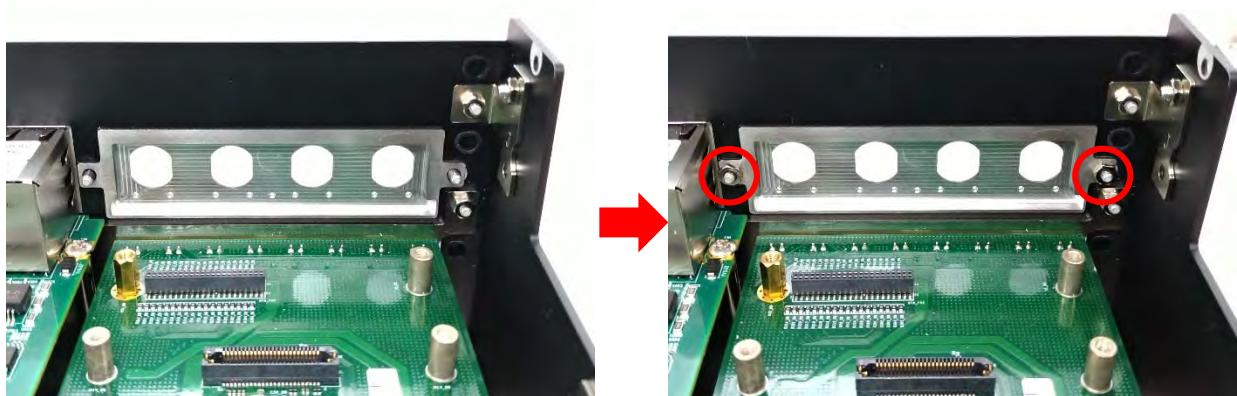
3. Locate the connector BTB\_FH1\_DB on DP-300 DTB.
