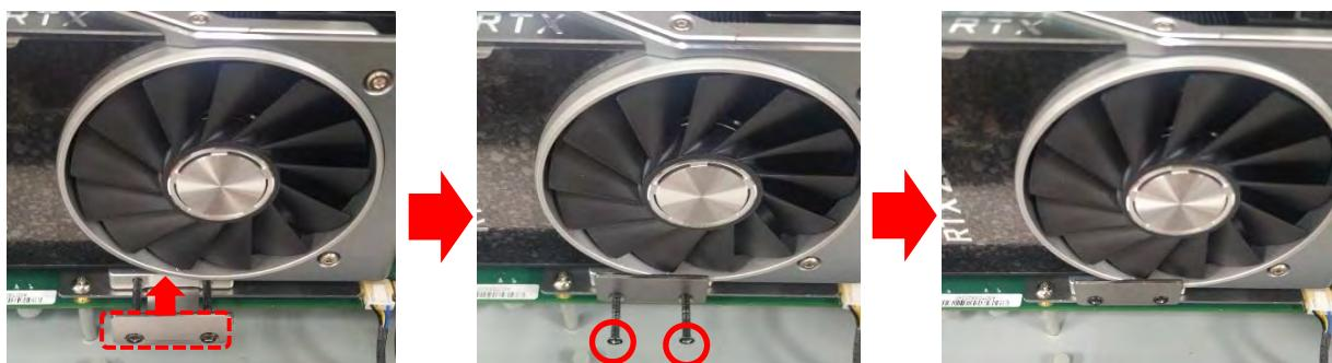
14. Fasten the screw (M3X6L) to fix the card retainer.
