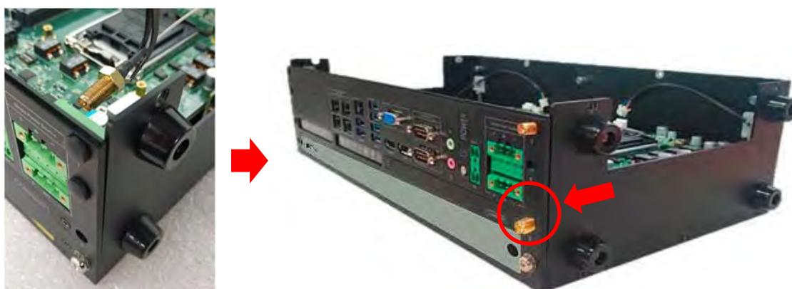
3. Put on the washer and fasten the nut of antenna jack.
