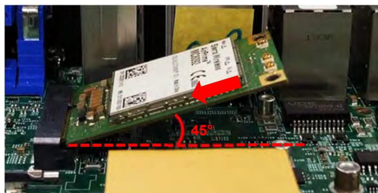
3. Press the card down and secure it with 2 screws.
