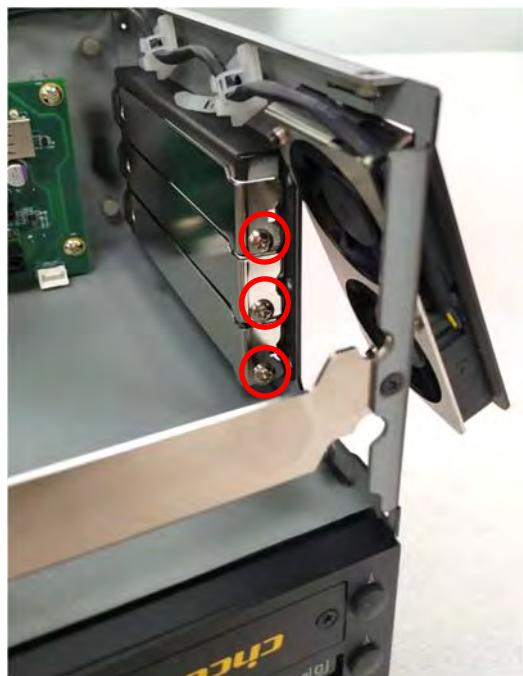
4. Loosen but not remove the four screws.
