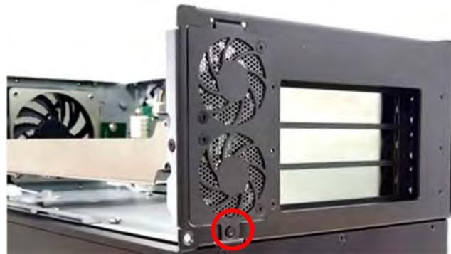
2. Press the wire and tape to close to the fan side, and then push out the fan seat.
