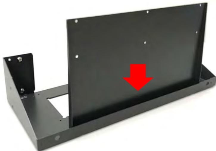
(4) Turn to the bottom side of the seat bracket. Fasten the four screws (M4X6L) to fix the back panel.
