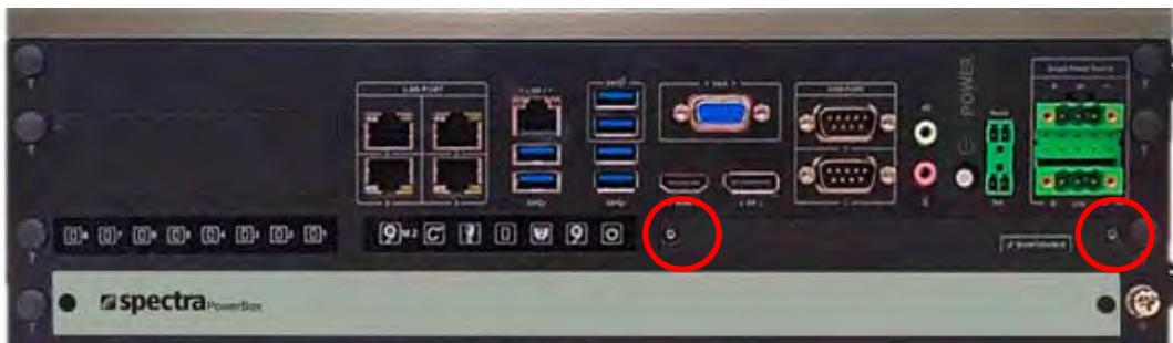
2. Locate the SIM card slot at front side and insert a SIM card into a SIM slot with the gold contacts facing down. Please pay attention to the insert orientation as illustrated.
