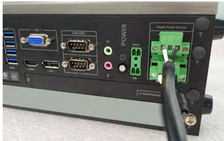
3. Fasten the four screws to fix the phoenix contacts.
