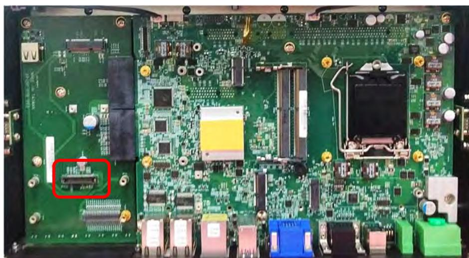
4. Aim the module's LAN ports at the holes on the bracket with an inclined angle, push it slightly and insert it vertically to the connector BTB\_FH1\_DB.
