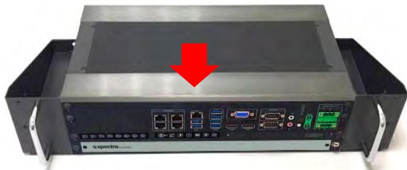
2. Turn to the bottom side of the 19" Rack Mount kit, and fasten the four screws (P4X5L).
