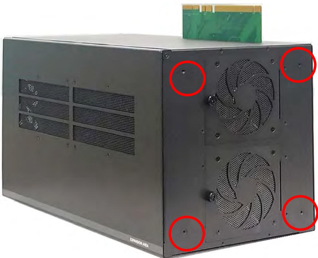
2. Attach on the two rubber foot pads and fasten the two screws to fix them.
