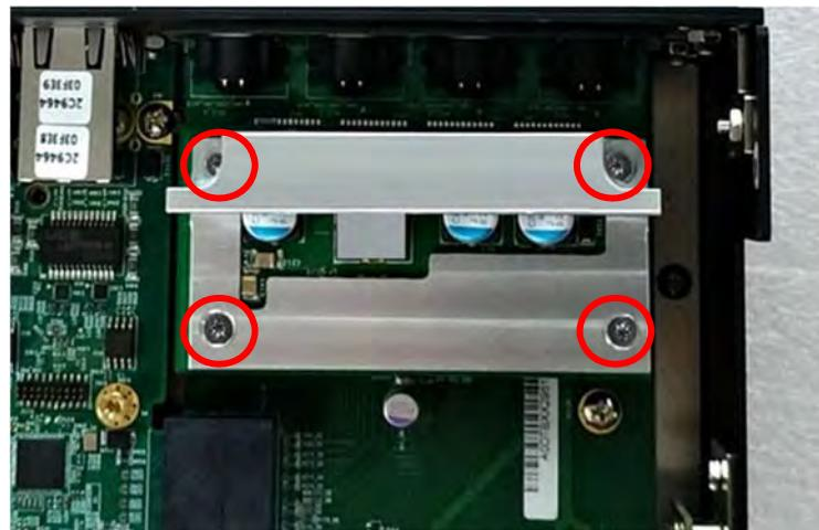
7. Paste the last two thermal pads onto the heatsink carefully, and then execute the step 8 in Chapter 6.2.2 to complete the installation.
