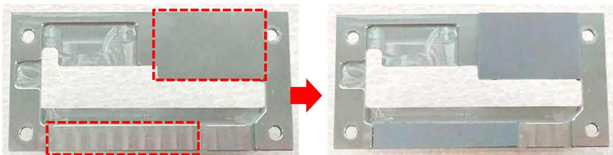
4. Paste a thermal pad on the choke.
