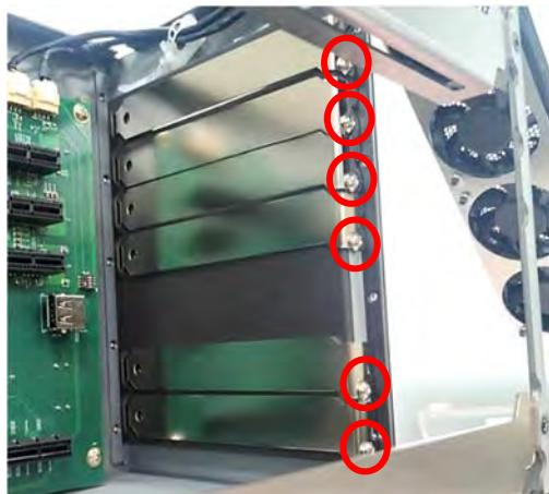
4. Loosen but not remove the four screws.
