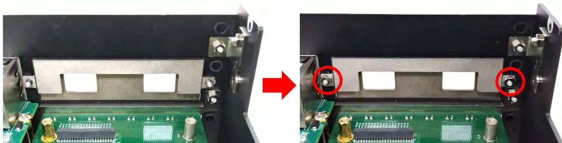
3. Locate the connector BTB\_FH1\_DB on DP-300 DTB.
