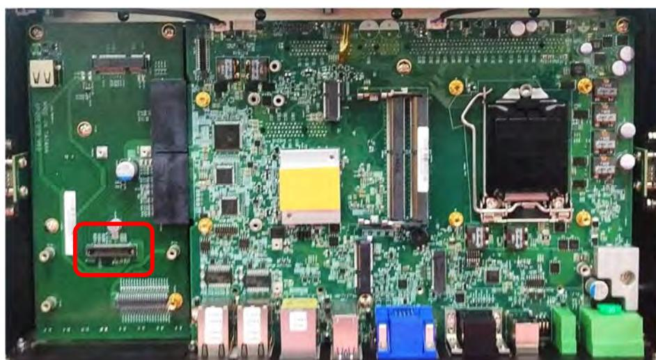
5. Penetrate the CMI-XM12LAN ports through the holes on the bracket.
