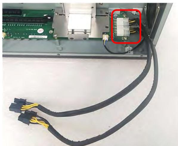
8. Insert the other ends of the two wires into the connector on the GPU card. The plug of the wire is a flexible design and can be connected to the 6-pin or 8-pin connector. (The picture shown below is just an example, the actual connection should be made according to user's GPU card.)
