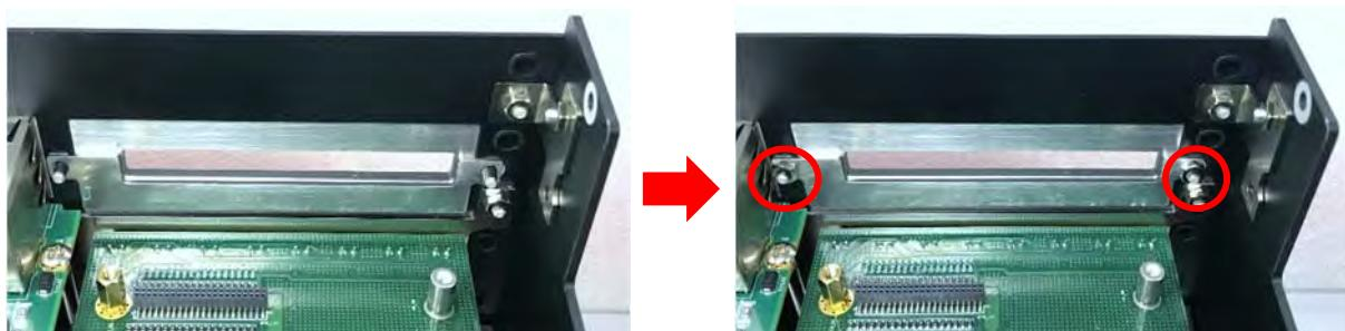
3. Locate the connector BTB\_FH2 on DP-300 DTB.
