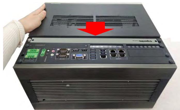
7.3 Keep holding the left side of the module's top panel, and press down the location on the panel as indicated.
