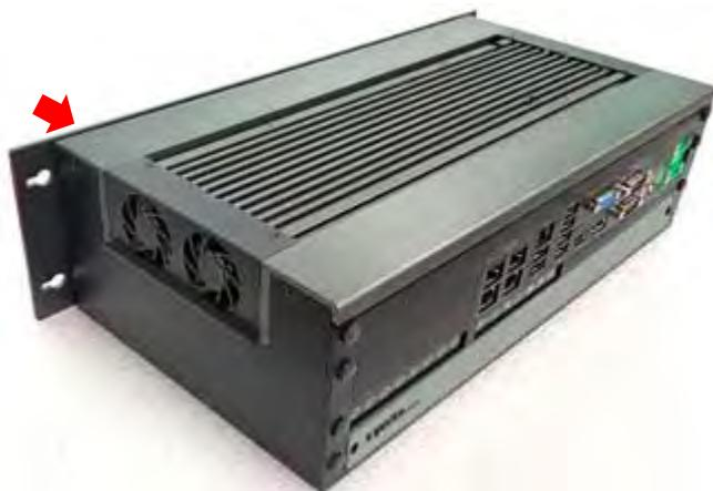
2. Use provided 6 screws to fasten the bracket.
