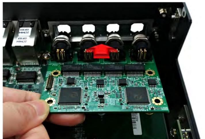
6. Push the CMI-M12LAN module slightly and insert it vertically into the connector BTB\_FH1\_DB.
