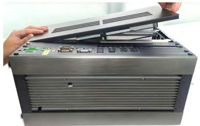
7.2 Keep holding the left side of the module's top panel, and press down the location on the panel as indicated.
