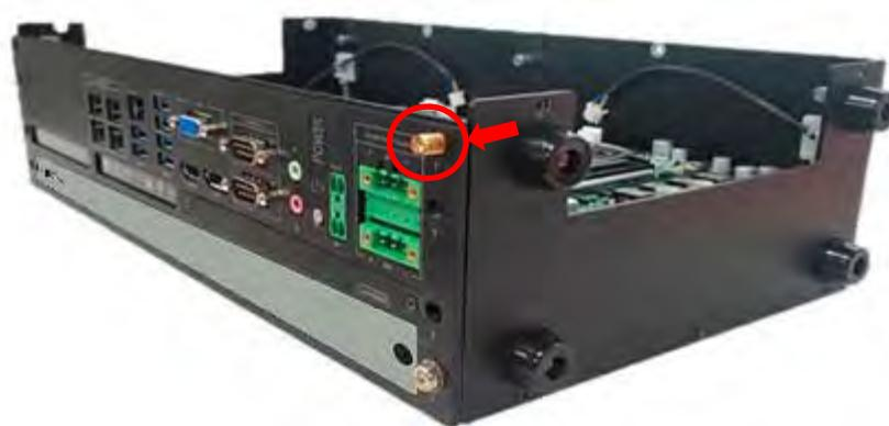
3. Put on the washer and fasten the nut of antenna jack.
