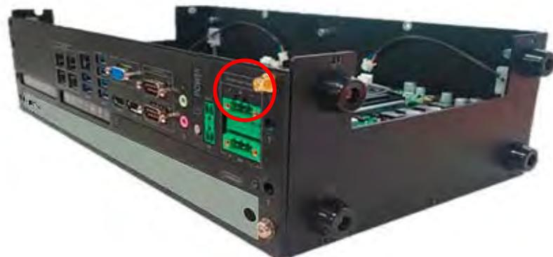
4. Assemble the antenna and antenna jack together.
