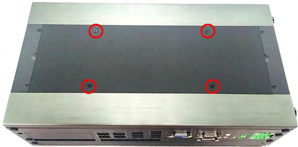
2. Loosen the 2 screws on the top cover.
