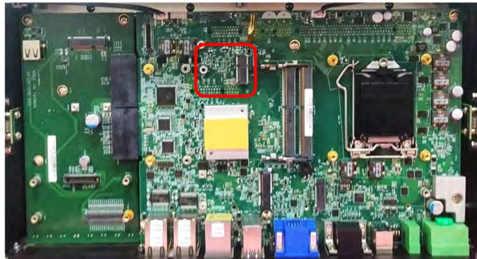
2. Tilt the M.2 E Key card at a 45-degree angle and insert it to the socket until the golden finger connector of the card seated firmly.
