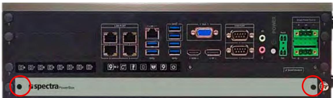
2. Loosen the screw(s) to remove the HDD bay cover bracket.
