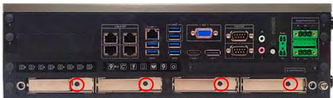
3. Pull the rotating arm and pull the HDD bracket out of system.
