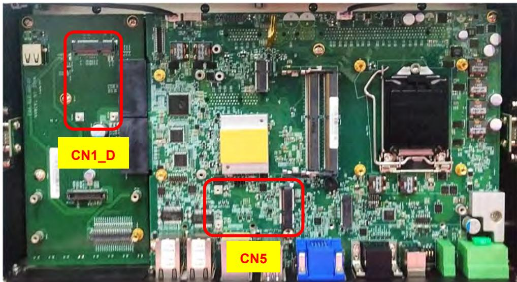
2. Tilt the Mini PCIe card at a 45-degree angle and insert it to the socket until the golden finger connector of the card seated firmly.
