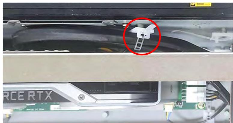
19. Press the wire and tape to close to the fan side and meanwhile push the fan seat back to the module. Fasten the screw and execute the installation step 7~8 in chapter 6.6.1 in the end.
