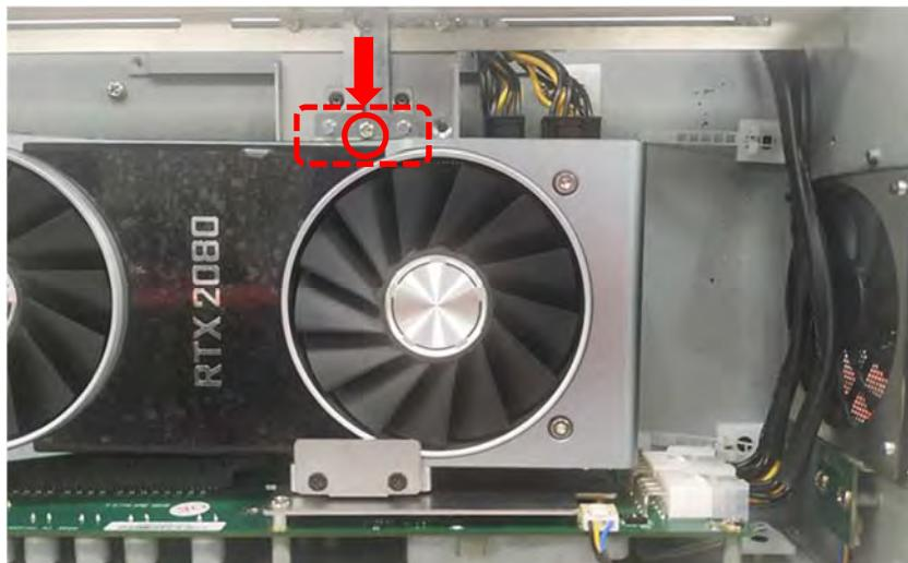
17. Fasten the screw (M3X5L).
