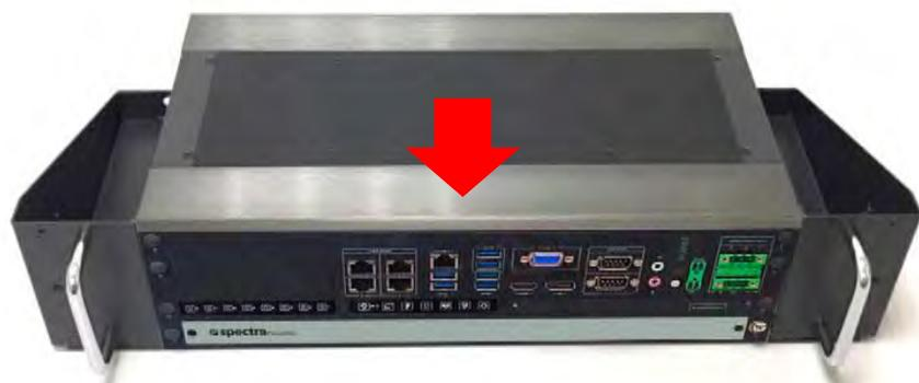
2. Fasten the four screws (M5X12) through the desk mount holes.
