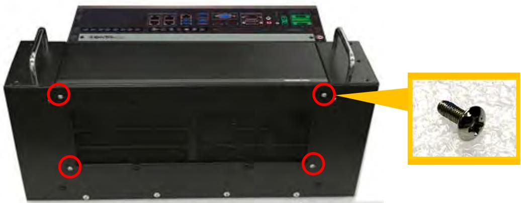
4. Turn to the back side of the 19" Rack Mount kit, and fasten the 6 screws (M4X6L).
