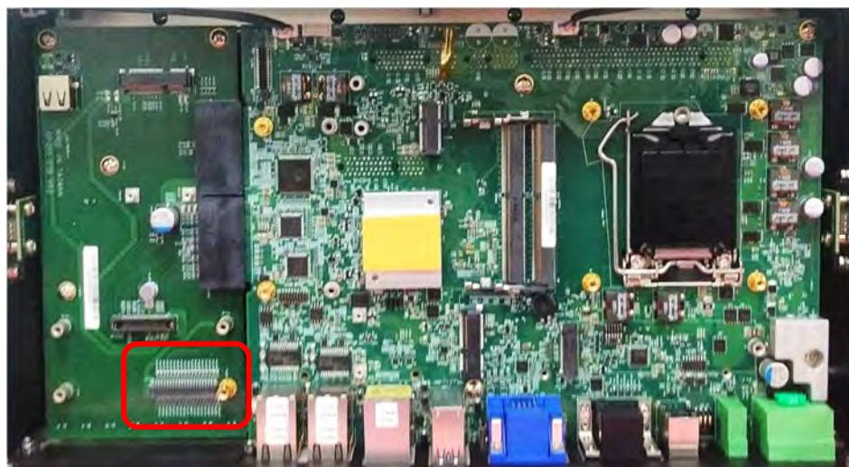
5. Penetrate the CMI-COM module through the holes on the bracket.
