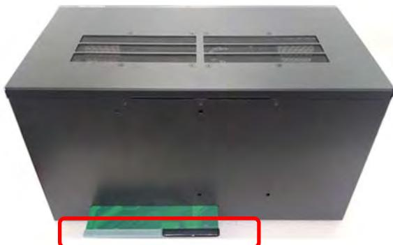
2. Loosen the screws on the panels of the module.
