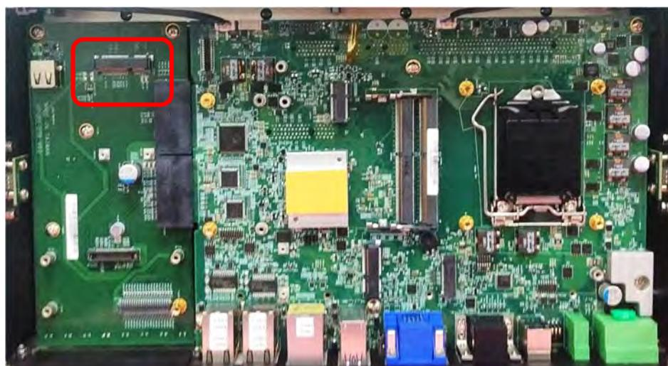
4. Tilt the Mini PCIe card at a 45-degree angle and insert it to the socket until the golden finger connector of the card seated firmly.
