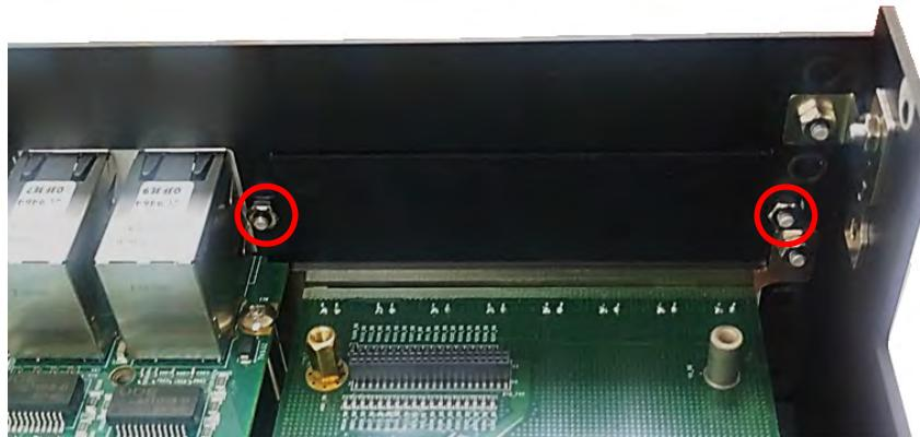
2. Attach the CMI-COM bracket, and fasten the 2 hex nuts to fix it as indicated.
