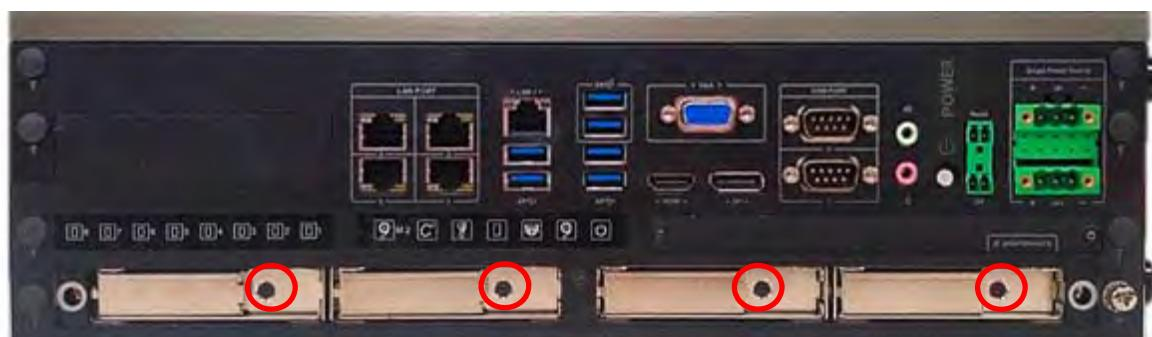
7. Fix the cover by fastening the two screws.
