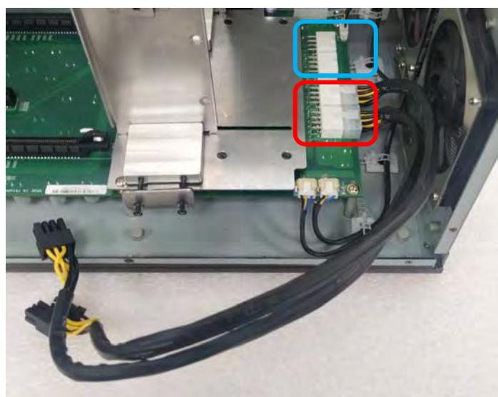
8. Insert the other ends of the two wires into the connector on the GPU card. The plug of the wire is a flexible design and can be connected to the 6-pin or 8-pin connector. (The picture shown below is just an example, the actual connection should be made according to user's GPU card.)
