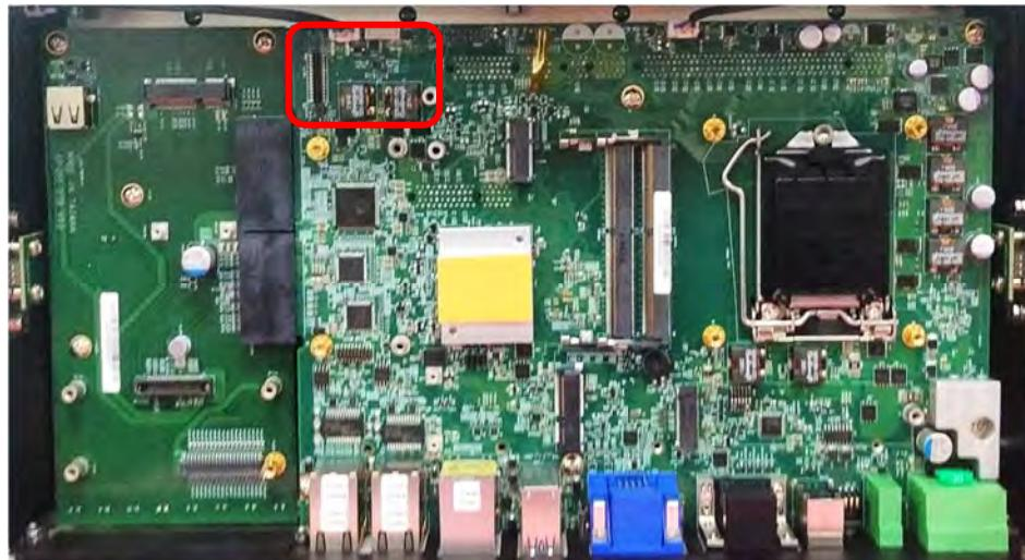
2. Insert the connector of IGN module to the female connector on system motherboard. (Make sure all the pins of IGN module's connector are firmly connected.)
