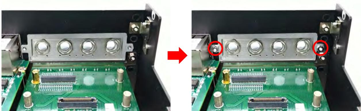
4. Locate the connector BTB\_FH1\_DB on DP-300 DTB.
