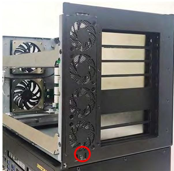
2. Press the wire and tape to close to the fan side, and then push out the fan seat.
