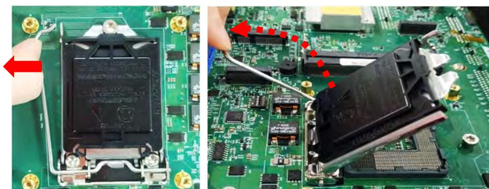
3. Align the notches on the CPU with protrusions on the socket. Hold the CPU by the edges and put on the CPU gently.
