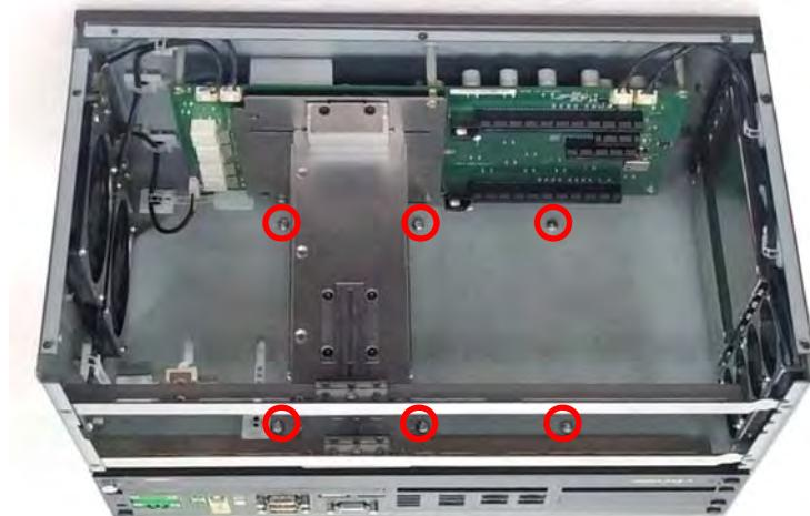
7. Assembling the top panel back to the module.
