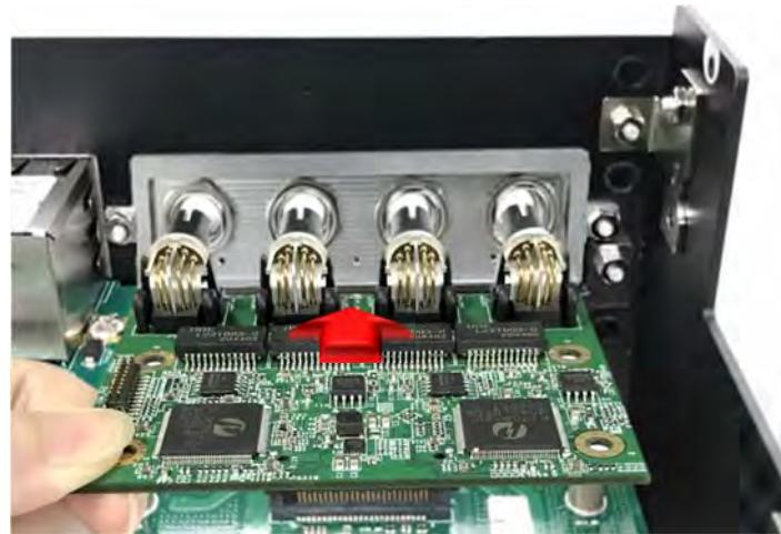
6. Push the CMI-XM12LAN module slightly and insert it vertically into the connector BTB\_FH1\_DB.
