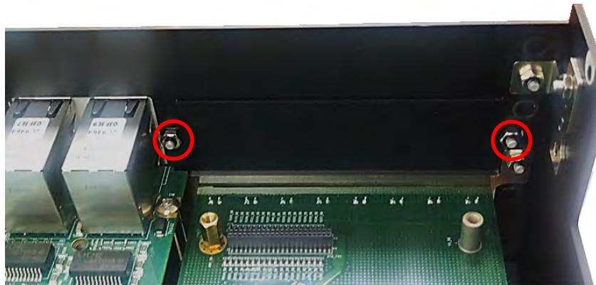
2. Attach the CMI-M12LAN bracket, and fasten the 2 hex nuts to fix it as indicated.
