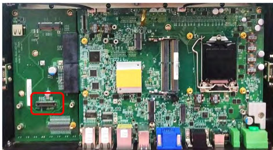
4. Remove the four hex rings from the CMI-M12LAN module.
