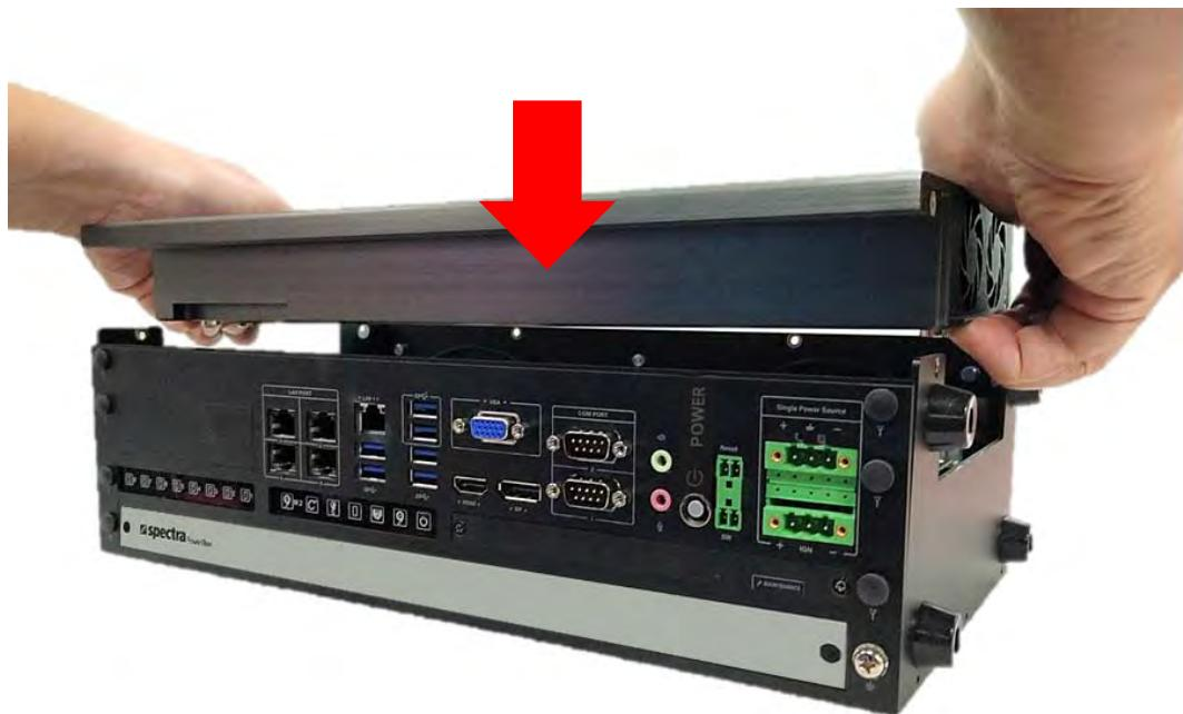
2. Fasten the 6 screws on the side and rear panel of the system.
