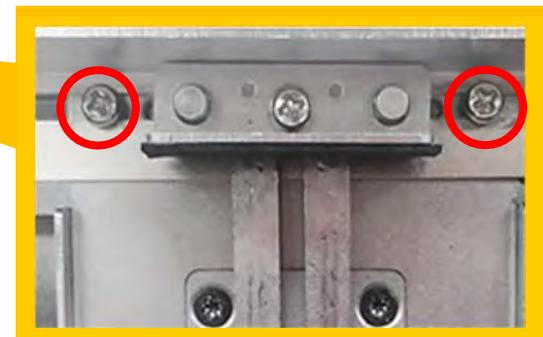
13. Push the plate till it contacts the GPU card, and then fasten the two screws to fix the GPU card.
