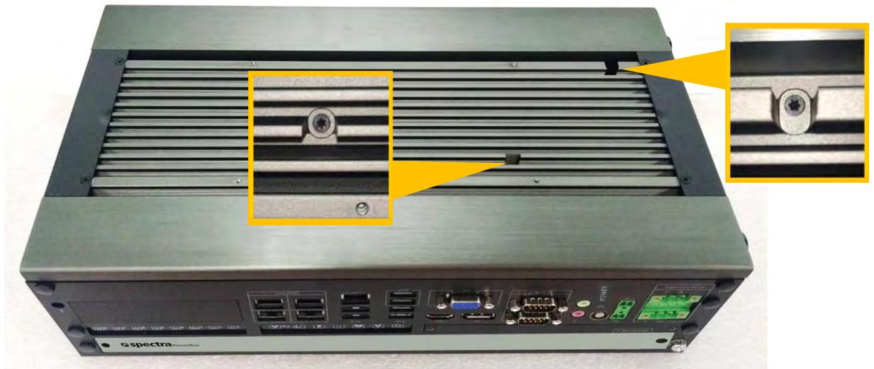
4. Put on the top plate, and fasten the 4 screws to fix the top plate.
