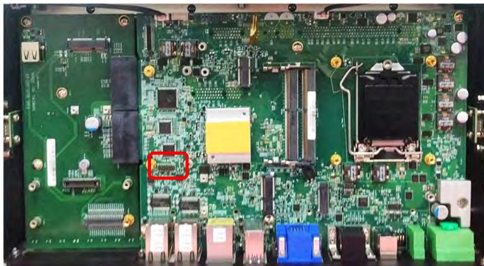
2. Insert the CFM-PoE module vertically into the female connector on the motherboard until it's connected firmly.
