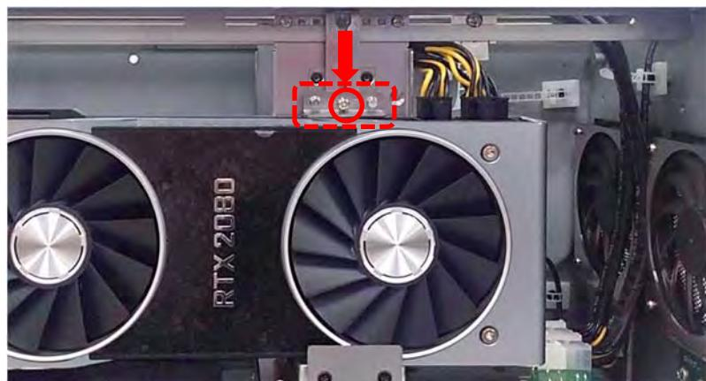
17. Fasten the screw (M3X5L).
