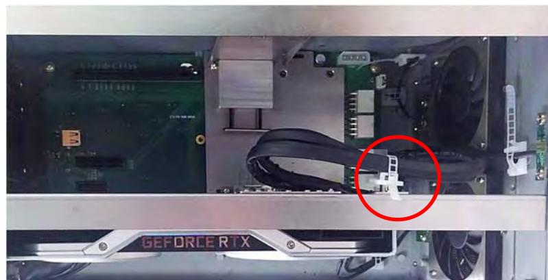
20. Press the wire and tape to close to the fan side and meanwhile push the fan seat back to the module. Fasten the screw and execute the installation step 7~8 in chapter 6.7.1 in the end.
