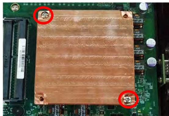
6. Place the thermal pad on the CPU heat sink.
