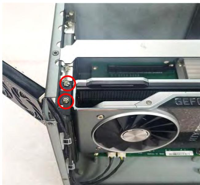
12. Fasten the four screws to fix the card retainer.
