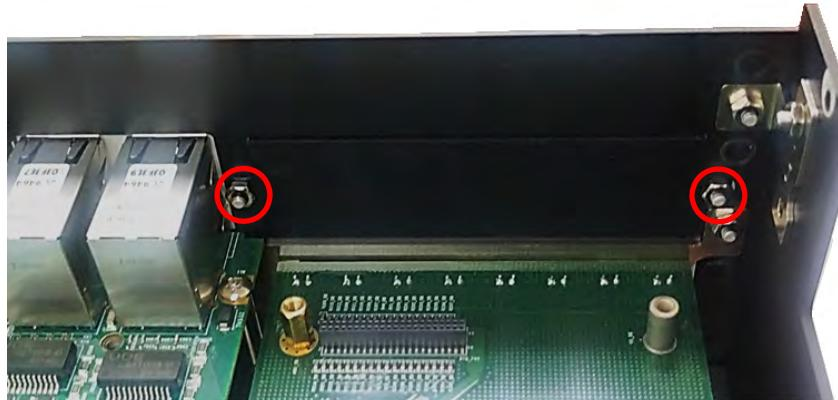
2. Attach the CMI-DIO bracket, and fasten the 2 hex nuts to fix it as indicated.
