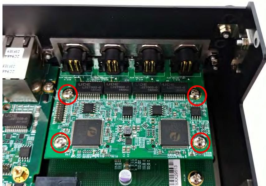
8. Fasten the four hex rings to fix the cover plate.
