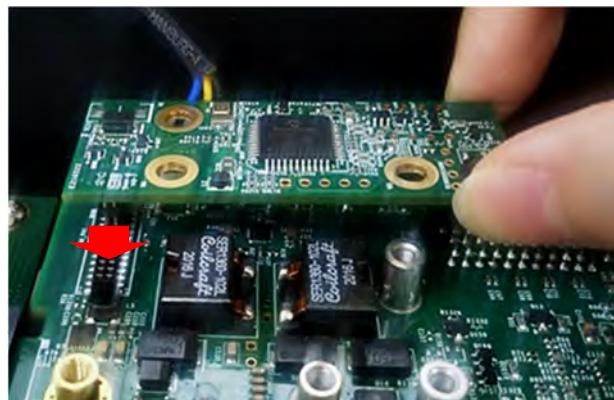
3. Fasten a screw to secure the power ignition board.
