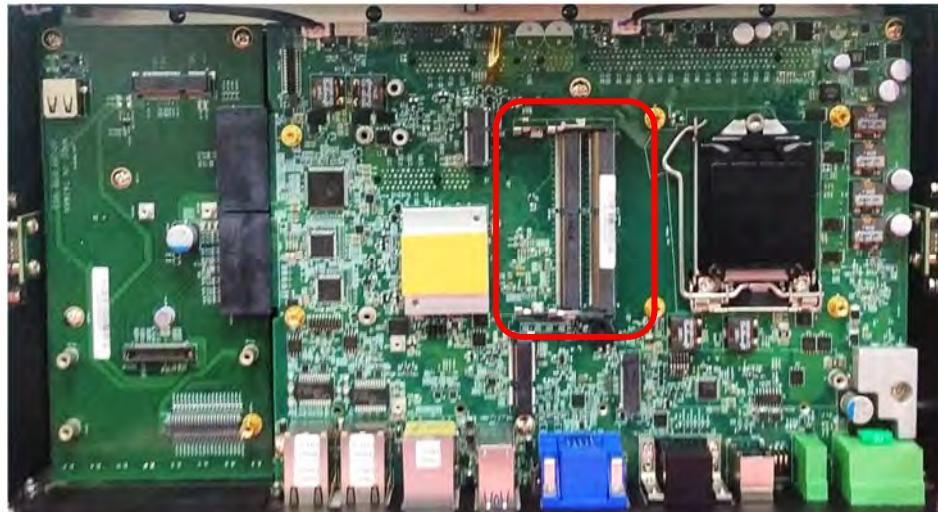
2. Insert a SO-DIMM at a 45-degree angle until its edge connector is connected to SO-DIMM socket firmly.
