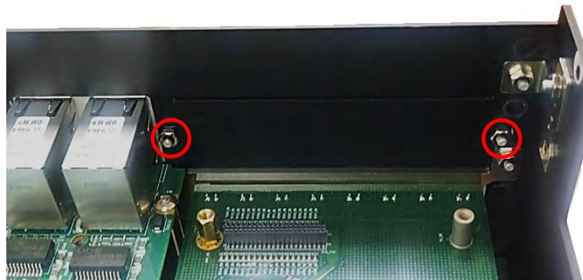
2. Attach the CMI-10GLAN bracket, and fasten the 2 hex nuts to fix it as indicated.
