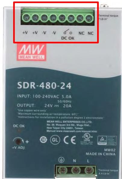
4. Connect the black wire to either “-V” socket, and connect the white wire to either “+V” socket.
