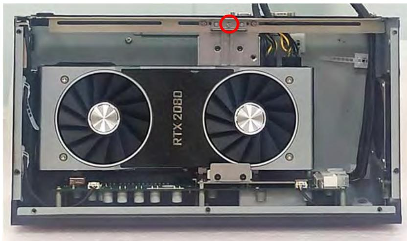
16. Make sure that the metal plate slides down until it touches the GPU card, and then fasten the screw to fix the GPU card.
