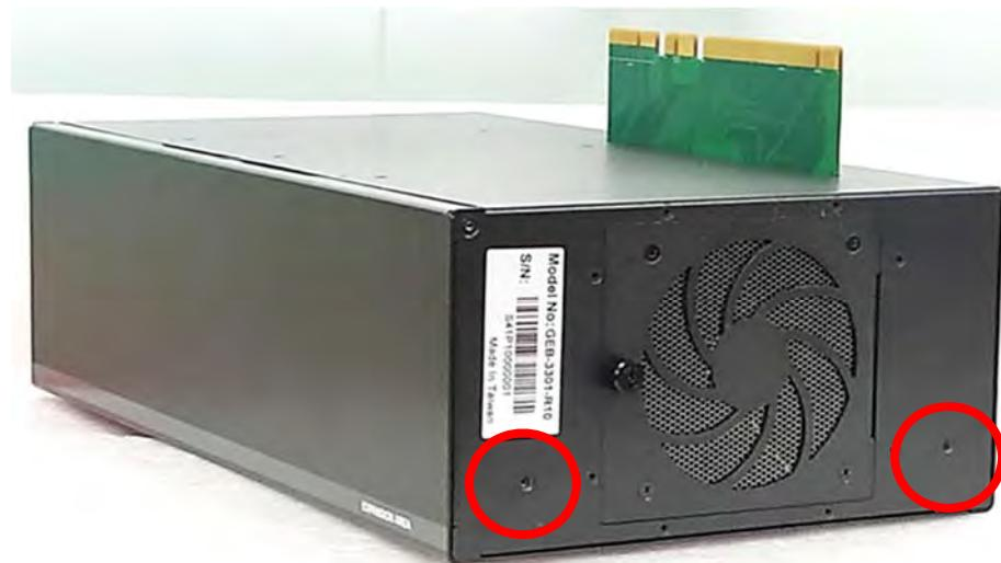
2. Attach on the two rubber foot pads and fasten the two screws to fix them.
