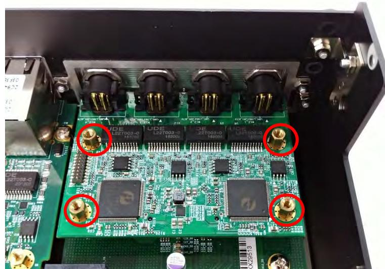
2. Insert the CFM-PoE07 module vertically into the male connector on the CMI module until it's connected firmly.
