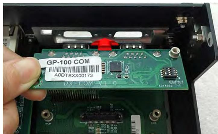
6. Push the CMI-COM module slightly and insert it vertically to the connector BTB\_FH1\_DB.
