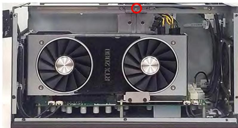
16. Make sure that the metal plate slides down until it touches the GPU card, and then fasten the screw to fix the GPU card.
