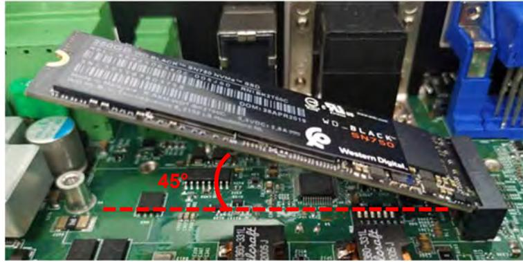
3. Press the card down and secure it with the screw.
