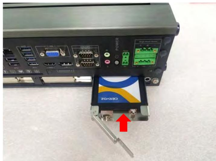
6. Place the rotating arm back and fasten the screw(s).
