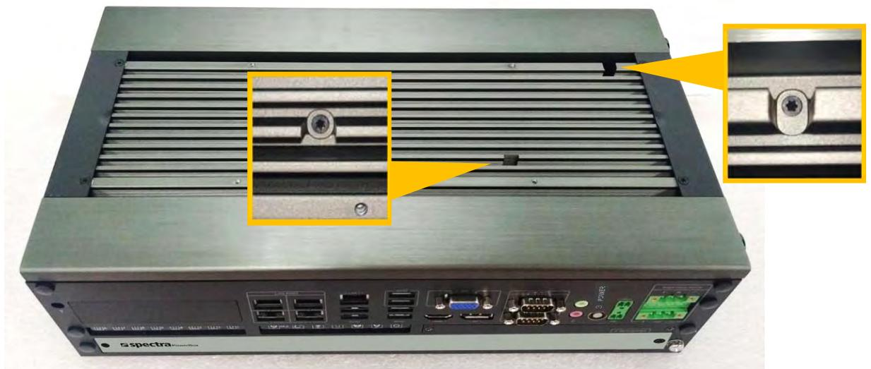
3. Loosen the 6 screws on the side and rear panel of the system.
