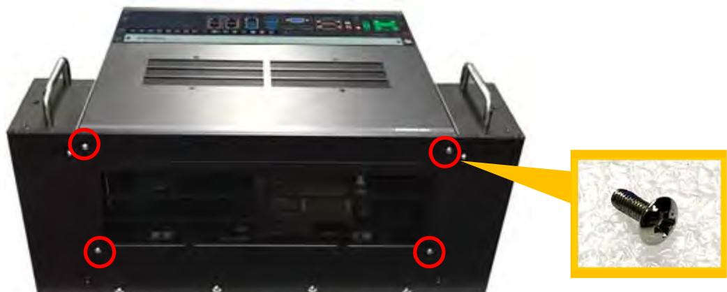
4. Turn to the back side of the 19" Rack Mount kit, and fasten the 6 screws (M4X6L).
