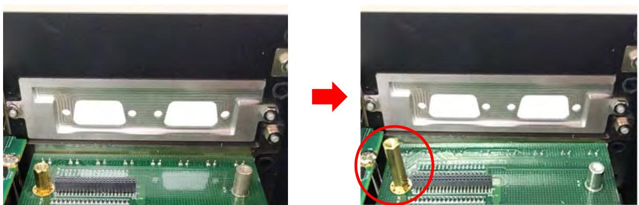
4. Locate the connector of BTB\_FH2 on DP-300 DTB.
