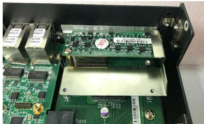
8. Fix the module and the metal board with the three screws.
