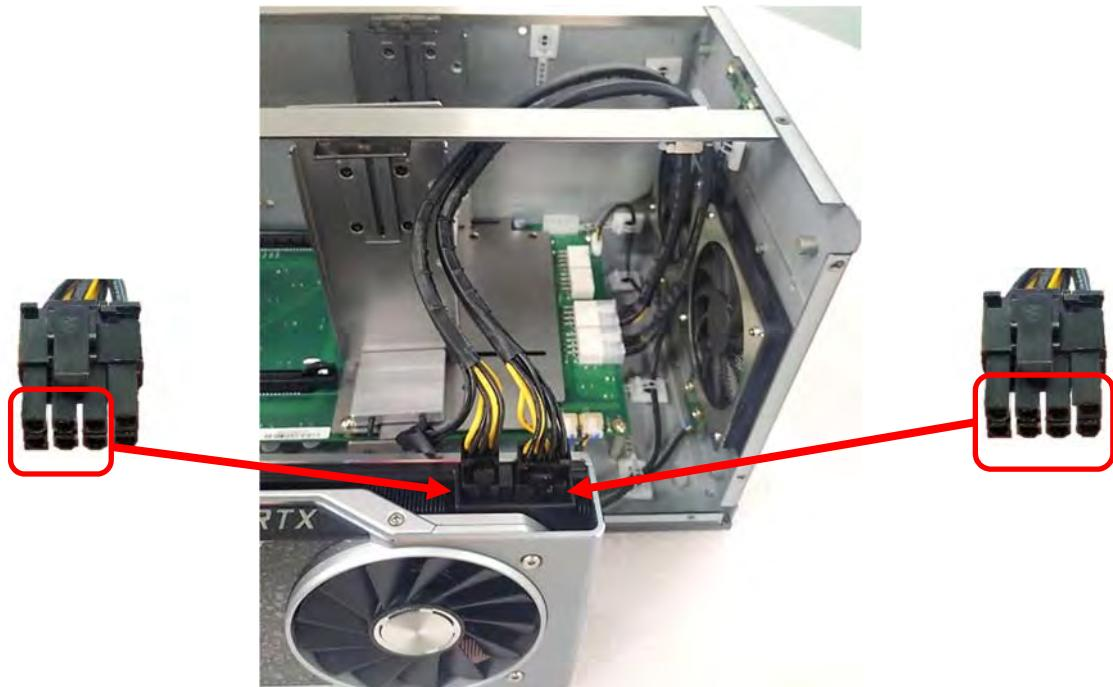
9. If there is exposed PCB on the GPU card which may touch the card retainer, please paste the black sponge bars on the lateral sides of card retainer before inserting GPU card into the module. If not, please skip this step and directly go to the step 10.
