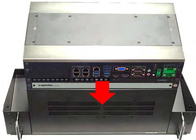
3. Turn to the bottom side of the 19" Rack Mount kit, and fasten the four screws (M3X8L).
