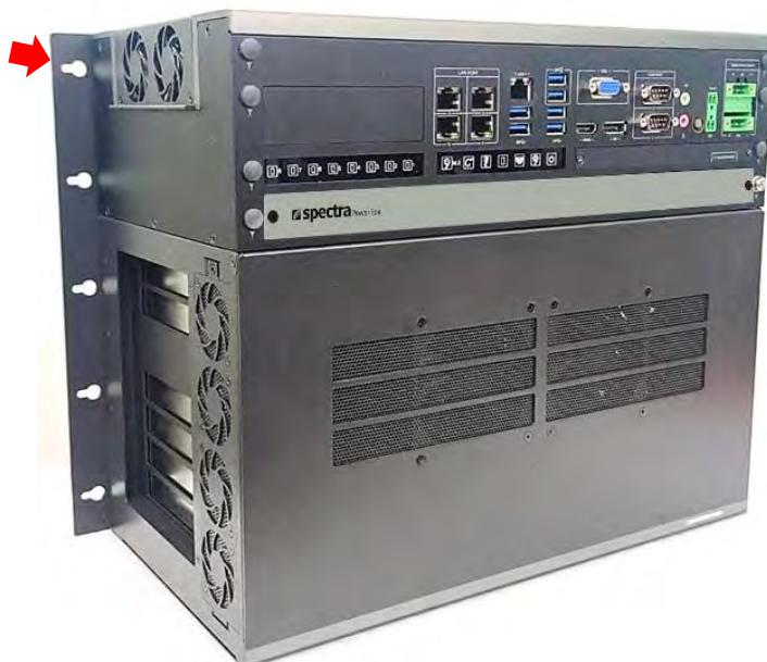
2. Use provided 15 screws to fasten the bracket.
