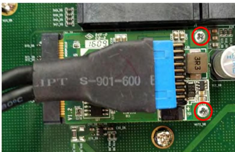
6. Attach the USB board to the back side of the cover plate.
