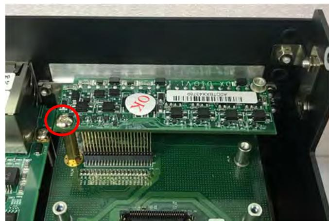
7. Put the metal board on the module as indicated.
