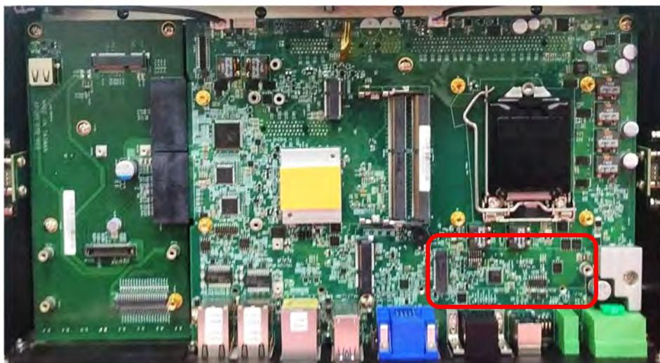
2. Tilt the M.2 M Key card at a 45-degree angle and insert it to the socket until the golden finger connector of the card seated firmly.
