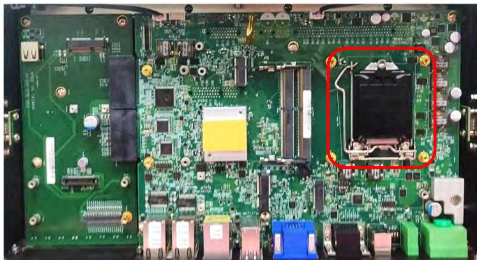
2. Pull aside and then lift up the socket lever to unlock the socket.
