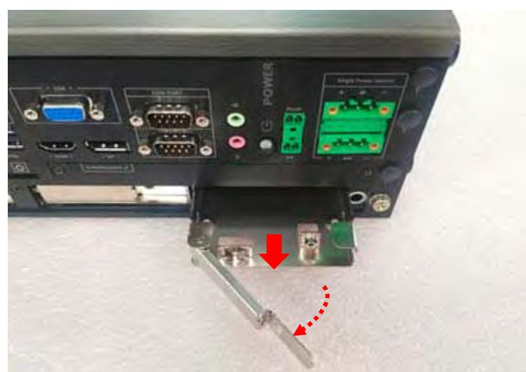
4. Make HDD bottom side face up, place the HDD bracket on it. Ensure the direction of bracket is correct and use 4 provided screws to assemble HDD and HDD bracket together.
