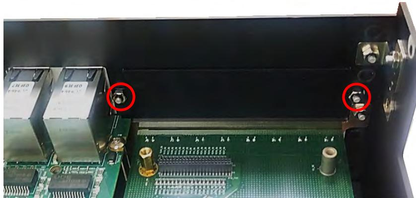
2. Attach the CMI-LAN bracket, and fasten the 2 hex nuts to fix it as indicated.
