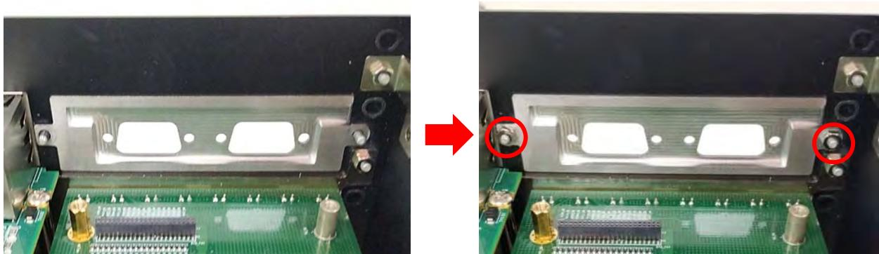
3. Replace the original copper pillar screw to the longer copper pillar screw as indicated.
