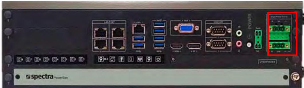
2. Aim the V- wire (black wire) at the V- port, and aim the V+ wire (white wire) at the V+ port on the DC\_IN connector. Then connect the phoenix contacts of the power supply to the DC\_IN connector.
