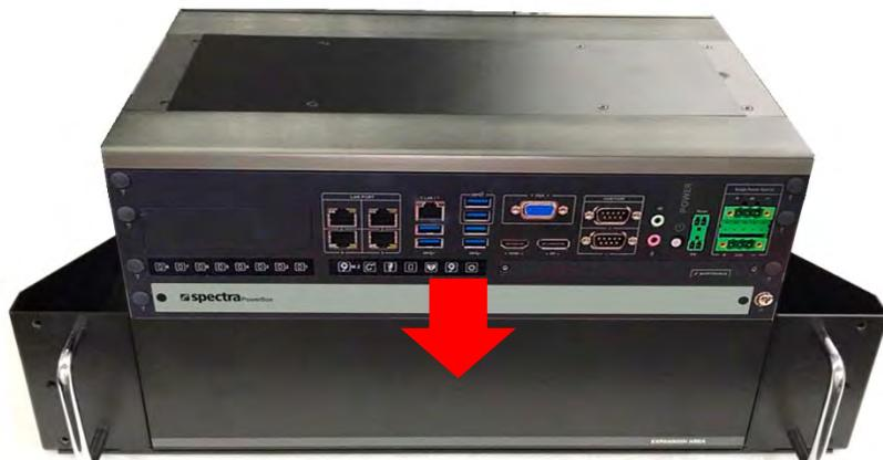
3. Turn to the bottom side of the 19" Rack Mount kit, and fasten the four screws (M3X8L).
