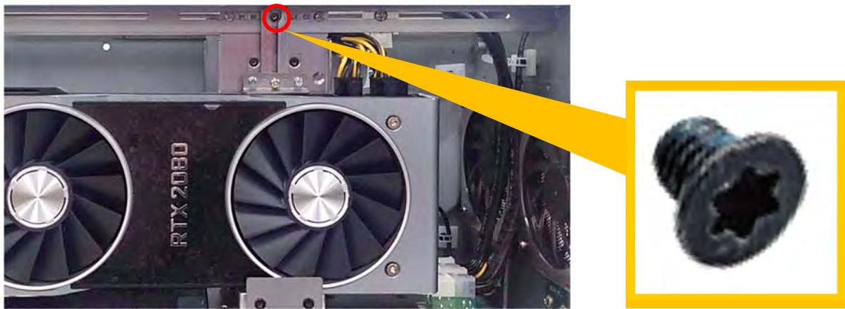
18. Loosen but not remove the screw in order to move the cable tie seat to an appropriate place.
