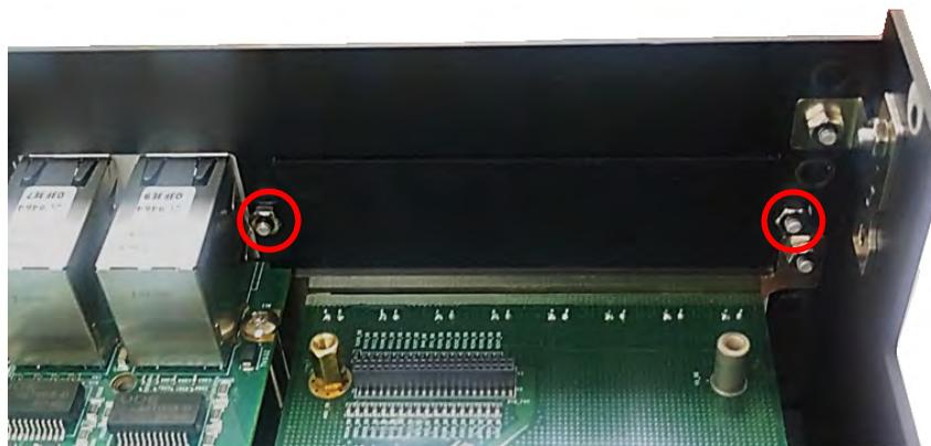
3. Attach the assembled M12 I/O bracket on to the system, and fasten the two hex nuts to fix it.
