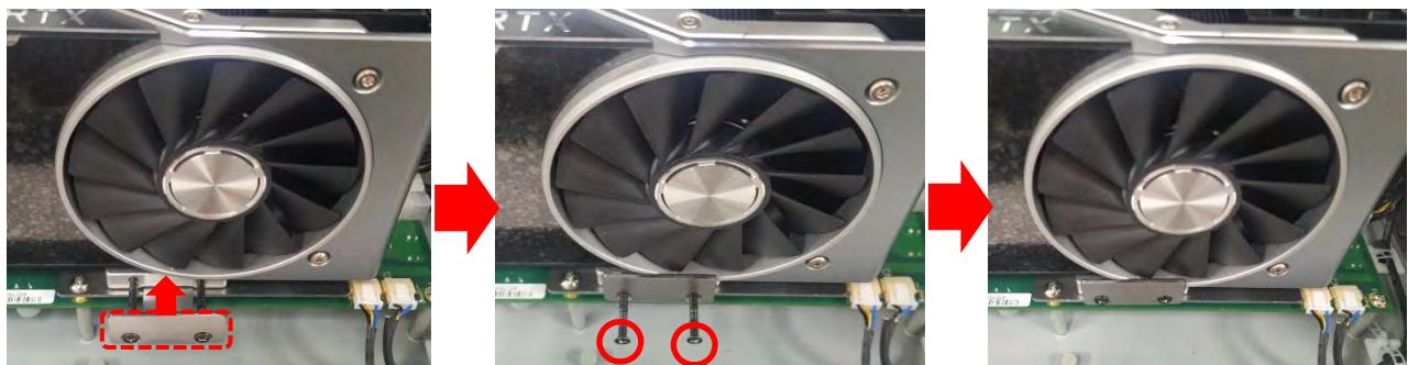
14. Fasten the screw (M3X6L) to fix the card retainer.
