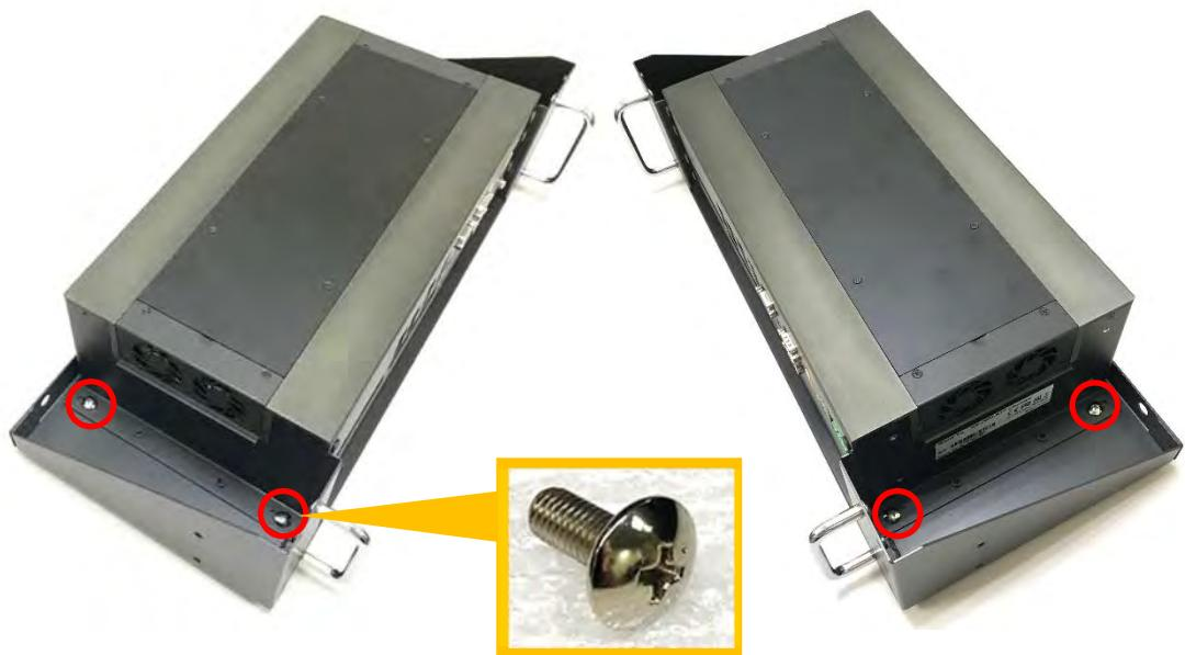
After complete the Method A or Method B steps, install the Spectra PowerBox 50 with the 19" Rack Mount kit onto the 19" Rack by fastening the 4 screws to complete the installation.
