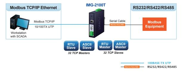
The advantage of having the IMG-210XT is to assist users to build an industrial environment between the Modbus TCP/IP Protocol and the Modbus RTU/ ASCII Protocol easily, thus offering an application solution to the industrial control equipment without Ethernet ports and the industrial control equipment can only control through an industrial PC workstation or industrial control panel.
