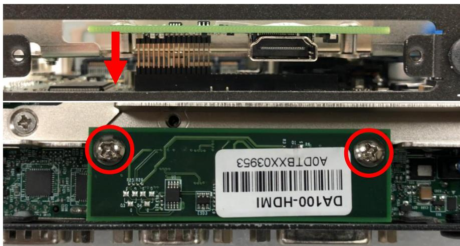
3. Attach the PB-100-HDMI bracket, fasten 2 screws as marked on photo.
