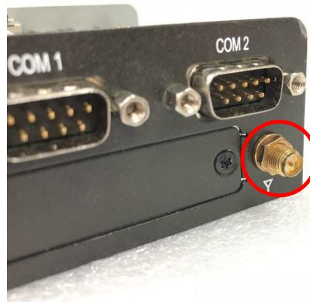
4. Assemble the antenna and antenna jack together.
