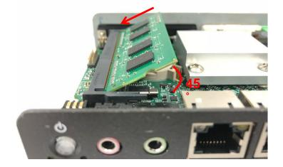
3. Press the module down until it's fixed firmly by the two locking latches on the sides.
