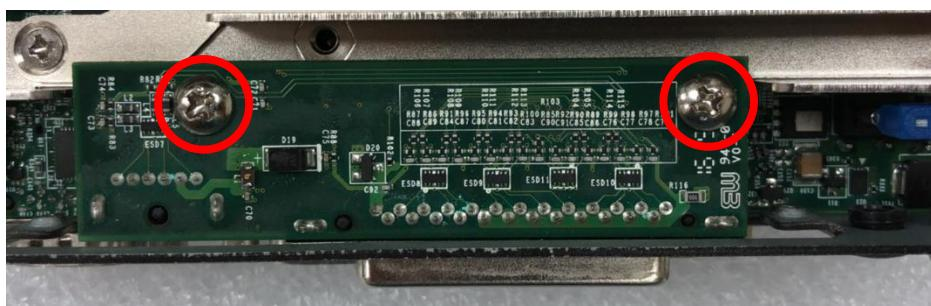
3. Attach the PB-100-LPT/PS2 bracket, fasten 2 screws and 2 D-Sub jack screws as marked on photo.
