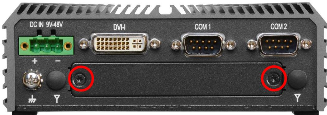
2. Insert PB-100-DP module vertically to the female connector on the system's mainboard, and fasten 2 screws to fix it.
