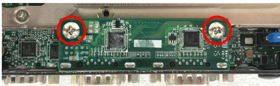
3. Attach the PB-100-COM bracket, and fasten 2 screws as marked on photo.
