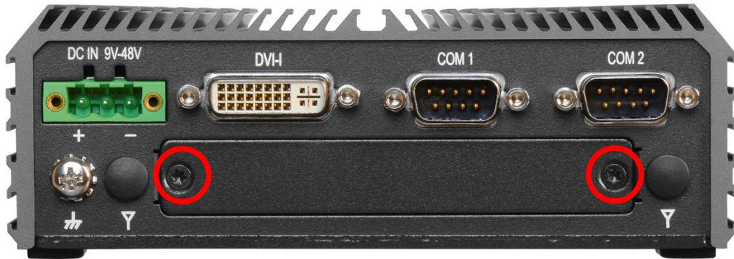
2. Insert PB-100-DIO module vertically to the female connector on the system's mainboard, and fasten 2 screws to fix it.
