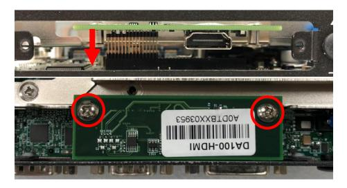
3. Attach the PB-100-HDMI bracket, fasten 2 screws as marked on photo.
