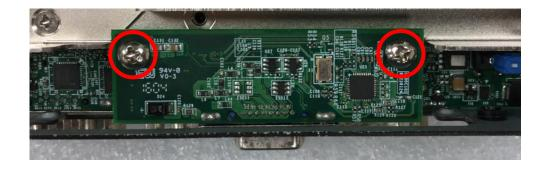
3. Attach the PB-100-VGA bracket, fasten 2 screws and 2 D-Sub jack screws as marked on photo.
