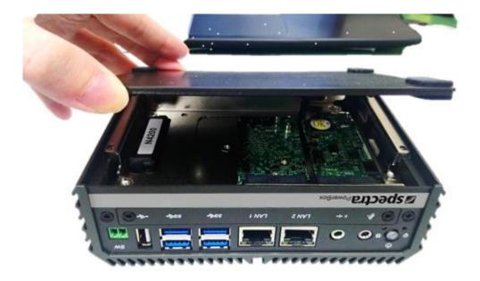
2. Fasten the 4 screws to fix the cover.
