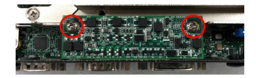
3. Attach the PB-100-DIO bracket, and fasten 2 screws as marked on photo.
