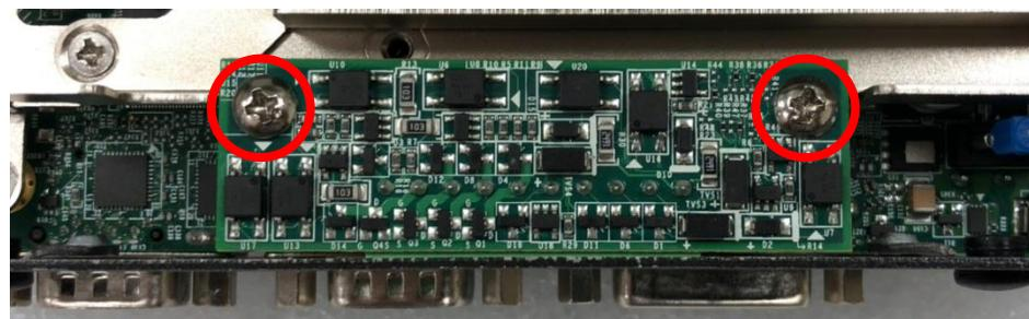
3. Attach the PB-100-DIO bracket, and fasten 2 screws as marked on photo.
