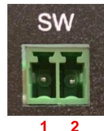
(Note: Please do not apply power to the pins. This port is used to connect a switch.)
