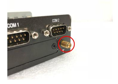
3. Put on washer and fasten the nut with antenna jack.
