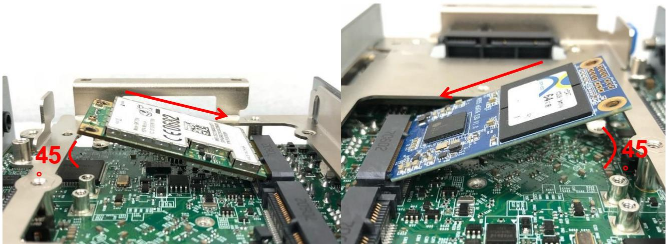
4. Press down the module and use the two screws to fix the module.
