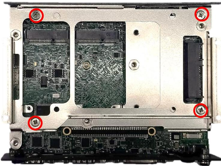
2. Make the PCB side of the HDD face up, place the HDD bracket on it. Ensure the direction of bracket is correct and use 3 provided screws to assemble HDD and HDD bracket together.
