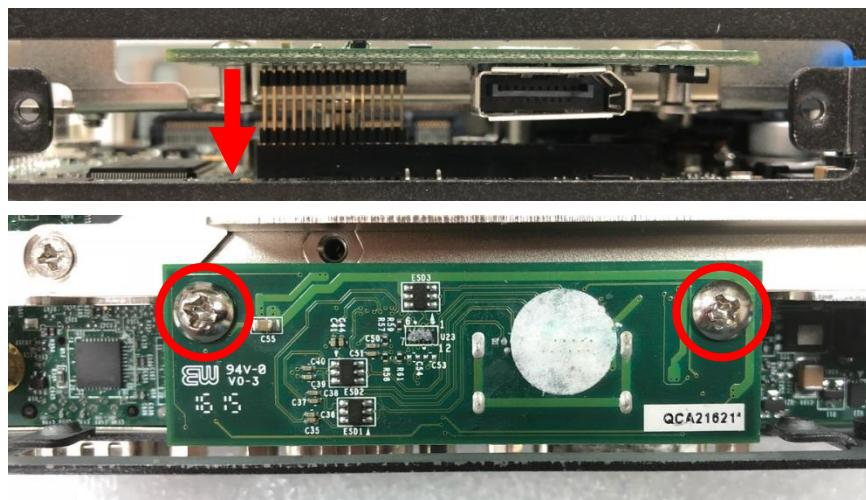
3. Attach the PB-100-DP bracket, and fasten 2 screws as marked on photo.
