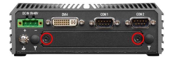
2. Insert PB-100-LPT/PS2 module vertically to the female connector on the system's mainboard, and fasten 2 screws to fix it.
