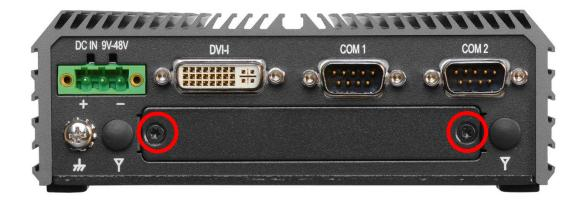
2. Insert PB-100-HDMI module vertically to the female connector on the system's mainboard, and fasten 2 screws to fix it.
