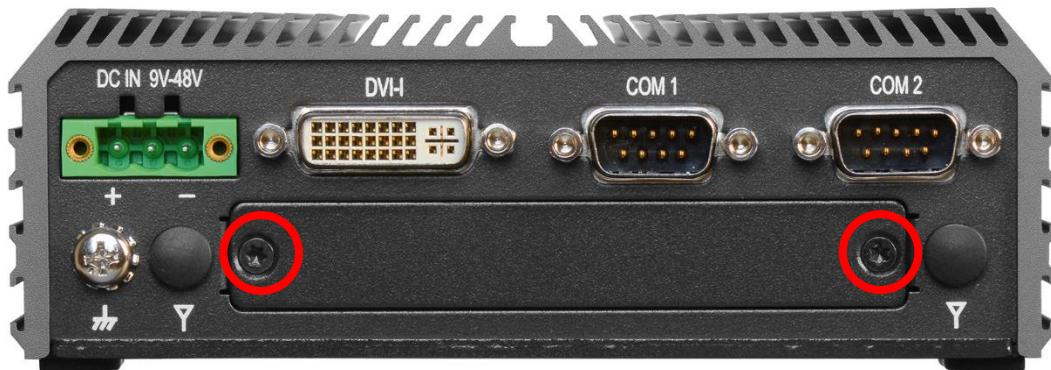
2. Insert PB-100-COM module vertically to the female connector on the system's mainboard, and fasten 2 screws to fix it.
