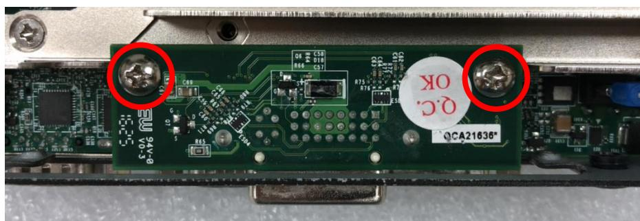
3. Attach the PB-100-DVI bracket, and fasten 2 screws as marked on photo.
