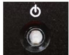
**AT\_ATX : AT / ATX Power Mode Switch**
