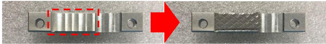
4. Paste the heatsink onto the CFM-PoE module carefully and fasten 2 screws to fix it.
