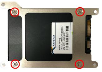
3. Turn over the HDD bracket. Connect the HDD bracket to the SATA connector of the unit and fasten the 4 screws.
