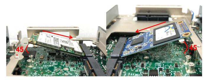
4. Press down the module and use the two screws to fix the module.
