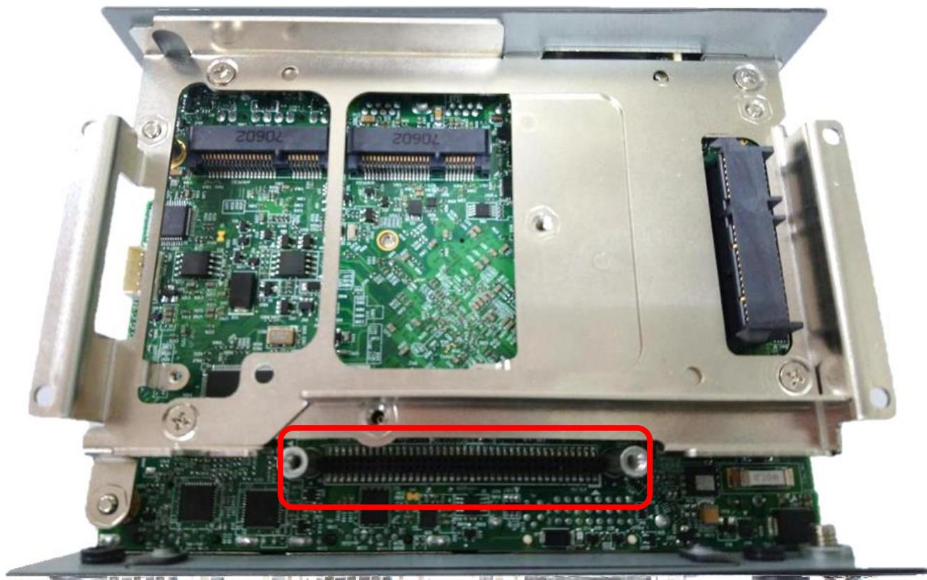
Locate the CMI connector on system motherboard as indicated.
