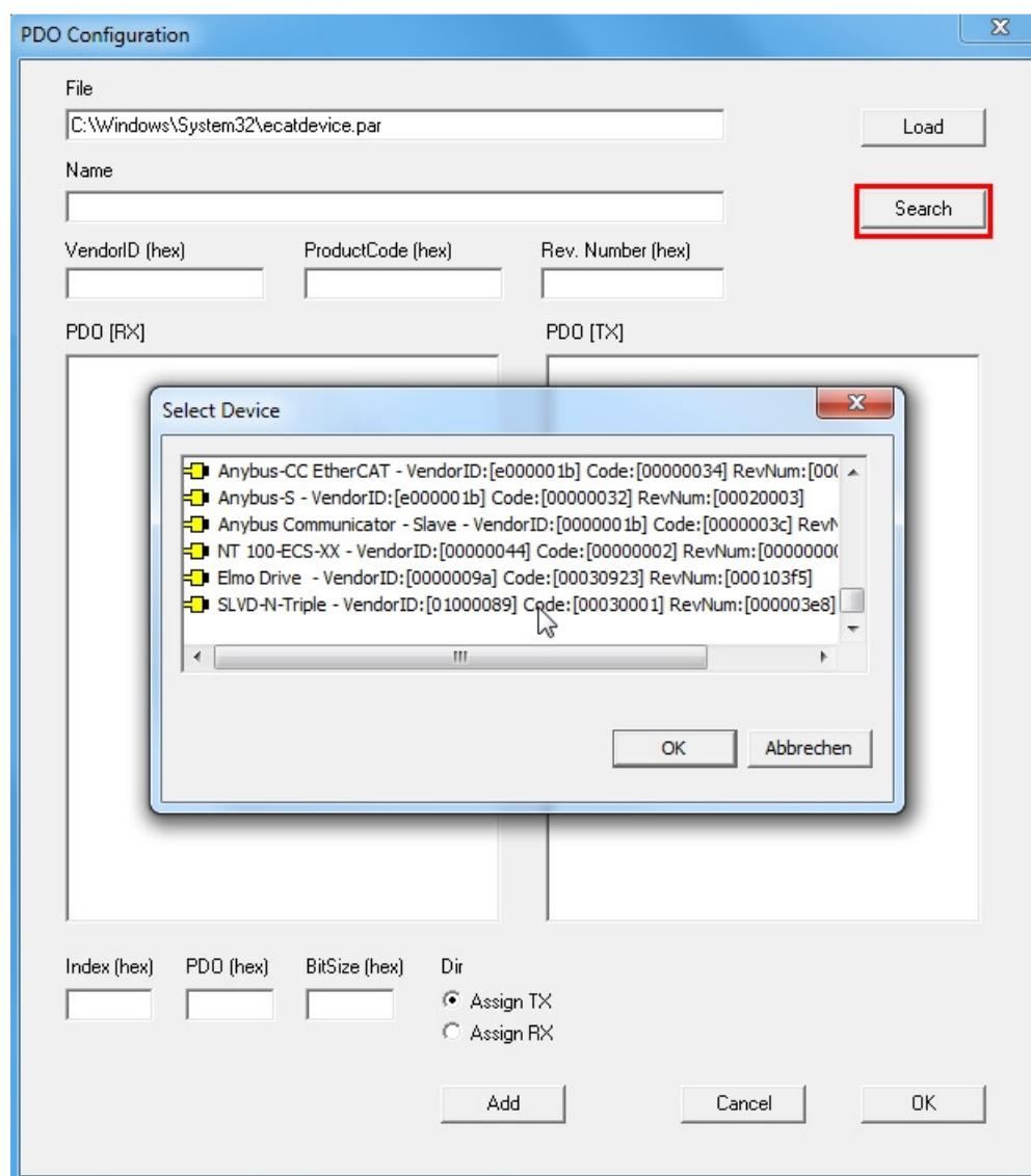
**Note:** Existing PDO-Mappings need to have an already listed PDO assignment (1C12 / 1C13). Otherwise the PDO mapping has to setup newly.
