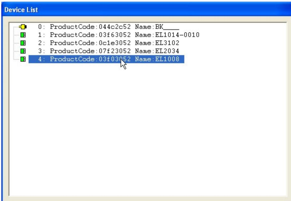
Note: With ECATVERIFY only the selected device will be enabled for further processing:
