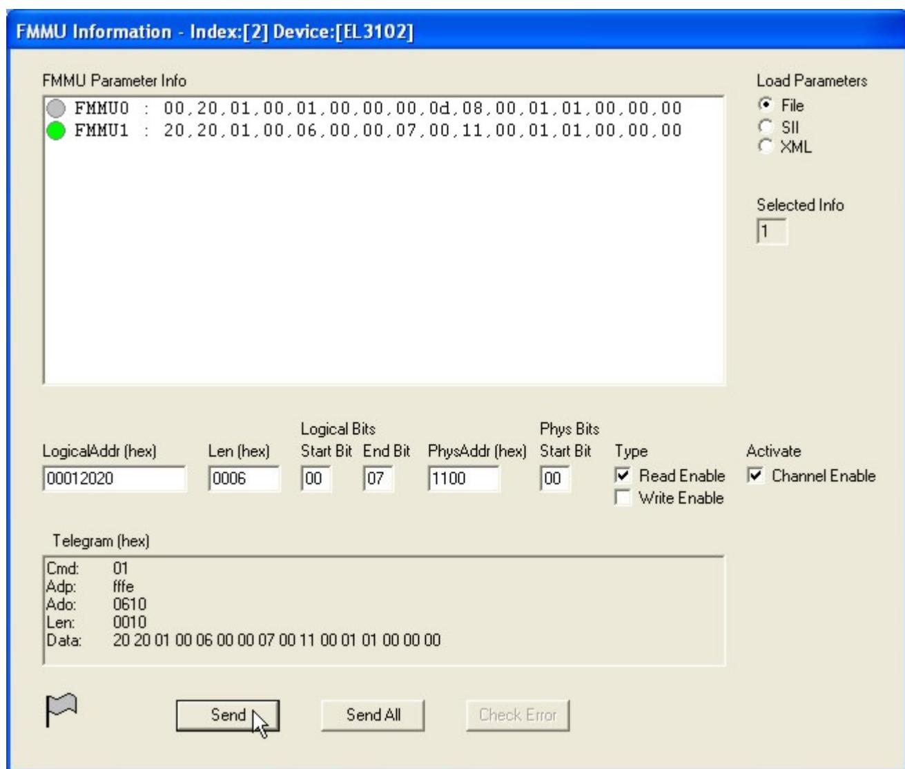
Each FMMU information can be selected by “Left Mouse Double Click” on the corresponding line. When the FMMU is selected it can be sent to the device. When all FMMU information is sent, configuration task is fulfilled. This configuration task uses the Library function(s), defined in ECATCOREDEF.H and SHAECATCORE.H:
