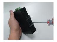
Step 1: Screw the DIN-rail on the Industrial Media Converter.
