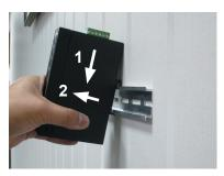
**Step 4:** To remove Industrial Media Converter from the track, lightly lift it up.
