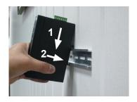
**Step 2:** Lightly slide the DIN-rail into the track.
