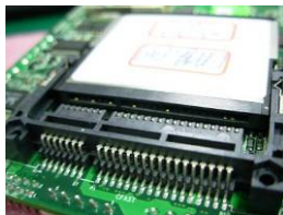
Installing the CFAST in the back of the board. Note that the slot direction and fool-proofing
