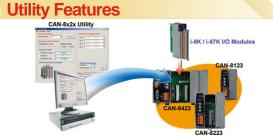
CAN-8x23 main unit can be plugged in the I-8K/I-87K IO modules to create a customized CANopen slave device and application. The CAN-8x23 Utility tool can configure the IO connection path, assembly and application objects information and create the EDS file of the device.
