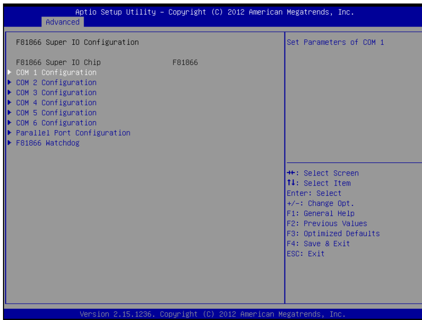
F81866 Super IO Configuration screen
